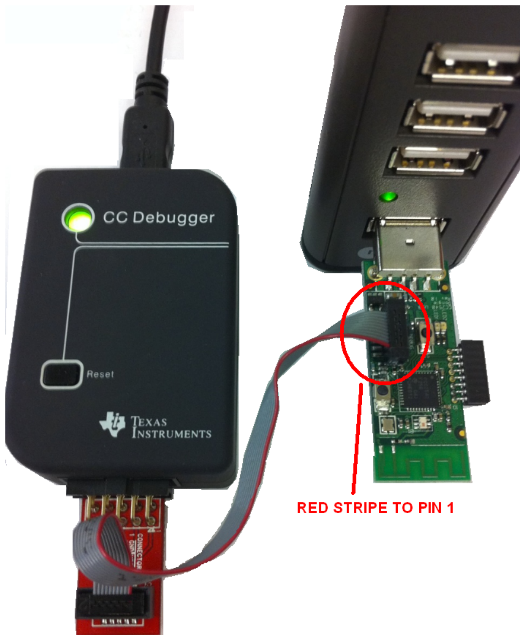
Figure 6-2. CC2540 USB Dongle Connected to CC Debugger
