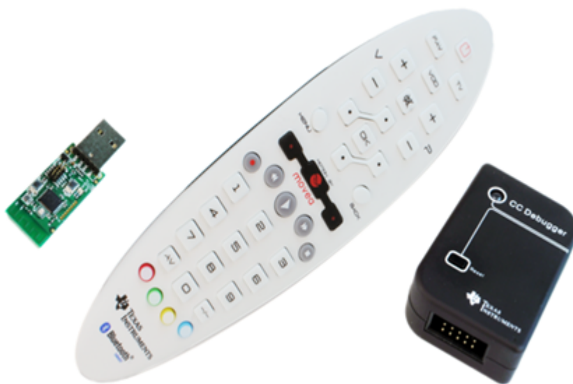
Figure 2-1. Hardware Included with the CC2541ARC
