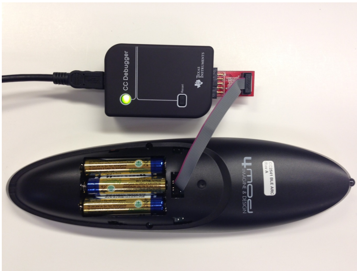
Figure 6-1. Advanced Remote Programming Setup
